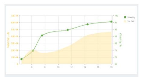
**FIGURE 9** A key function of CellarMate is its ability to increase the viability of the cells during the preparation of a starter culture. Starting at an average viability of 68%, from hydration to 18 hours later, the culture has reached 96% viability and is ready to pitch.
