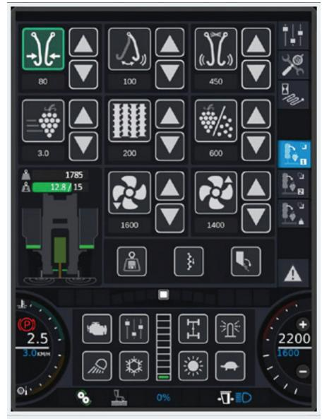
**FIGURE 6** The Harvester Management Instrument controls many functions of an over-the-row harvester such as speed, amplitude and force of the beater bars, harvest weight and targets.
