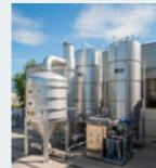
DESCRIPTION: Thermovin allows the production of ready-to-drink wines with bright, deep violet red colors, a fragrant aroma, smooth and velvety taste and is high energy saving with a limited footprint and full automatic handling and CIP. The Sonitus—ultrasound technology applied to red and white grapes in order to increase color and aromas extraction from skins—requires just a few minutes of treatment and features low operating
