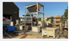
standard ROTOVIB with single roller sorters. The functionality of the second roller sorter is to eliminate the small MOG (seeds, shot berries, rot, etc.) by utilizing a tighter array of rollers that will allow the very small waste to pass through and the good berries to discharge.
