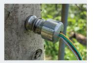
status, known as water potential. Because the measurement is taken directly inside the water-carrying tissue, readings are very accurate and reliable. No other sensor can provide real-time, 24/7 accurate water potential measurement.
