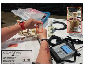
FIGURE 2 The NomaSense P300 DO meter uses luminescence to test oxygen in the headspace without popping the cork.
