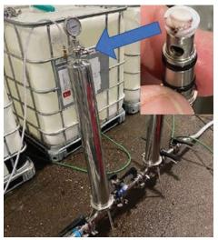
FIGURE 3 Damaged bleeder valve
