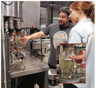
**FIGURE 5** Smith and Neely take note of excessive foaming post-filling.
