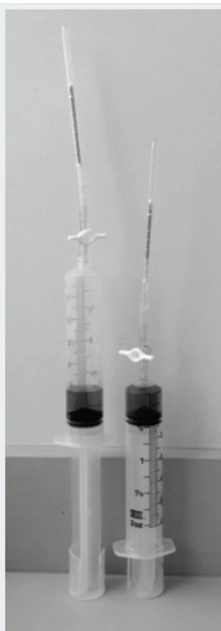
FIGURE 2 The headspace gas detection tube apparatus prior to (left) and after (right) headspace expulsion through the gas detection tube.
